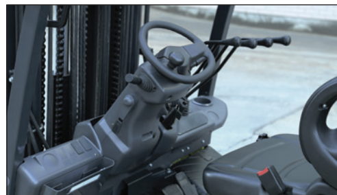
Adjustable steering column according to operator's preference to reduce fatigue.
