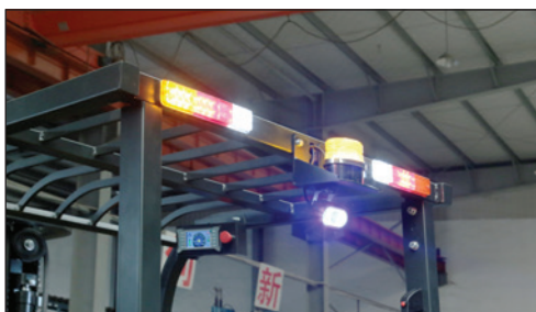
Blue spot light: reminding pedestrians when reversing.
