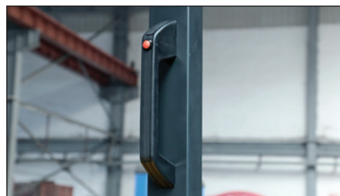
Back-up handle with horn button: improving both driver's comfort and reversing safety.
