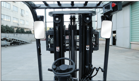
Wide view mast offers good driving vision.
