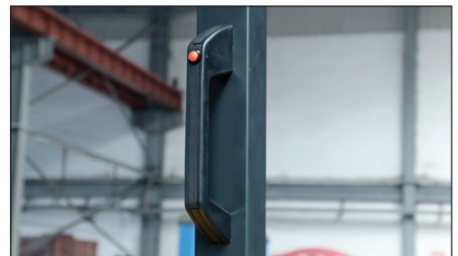
Back-up handle with horn button; improving both driver's comfort and reversing safety.
