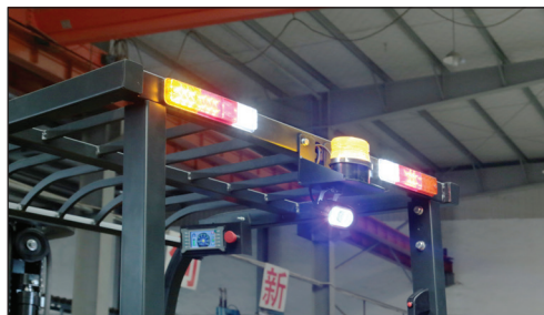
Blue spot light: reminding pedestrians when reversing.
